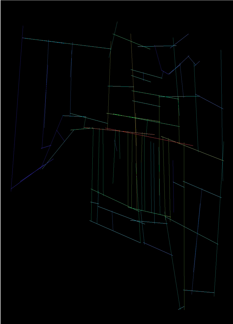
Map 8 Axial integration map of Miskolc-Gordon representing the late 19th century situation – The scale runs from red to blue, with red indicating high level of axial integration and blue referring to low. (Created by Zoltán Bereczki)
